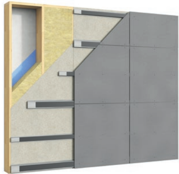
Light wall with horizontal VFL steel profiles
